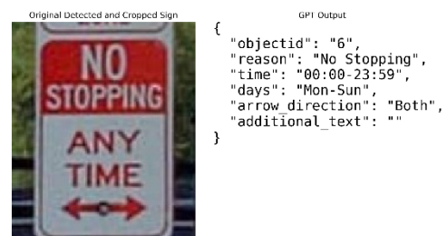
Figure 12: Successfully detected and cropped sign passed into GPT4.0, with respective response.
